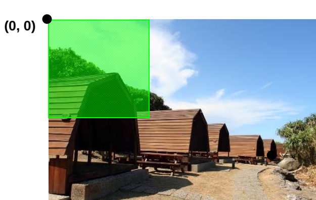
Figure 4-51 : Source0 is Layer1[(0,0) ~ (199,199)] ,Source1 is Layer2[(0,0) ~ (199,199)], executes alpha blending and showing on Destination Layer1[(0,0) ~ (199,199)], alpha = 16.
